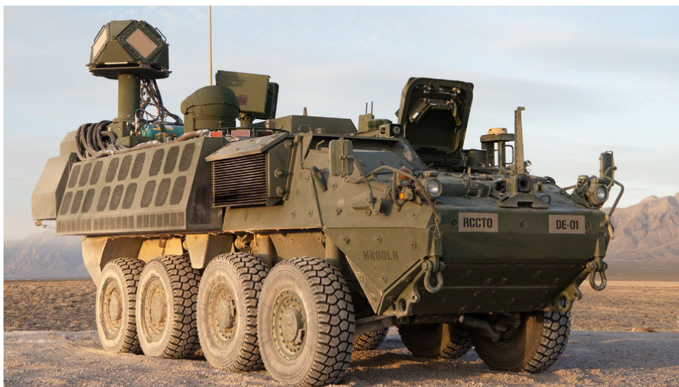
Figure 4 – Directed Energy Maneuver-Short Range Air Defense mounted on a Stryker armored vehicle
