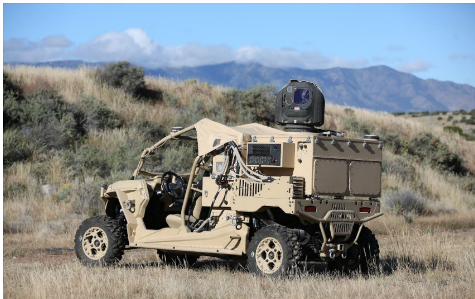
Figure 3 – High-energy laser weapon system mounted on a Polaris MRZR vehicle (dune buggy)
